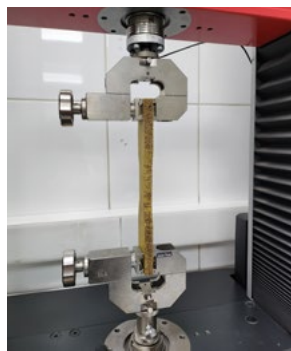
FIGURE 7. Tensile tests. The trials confirm the material's dimensional stability and resistance under tensile loading.
