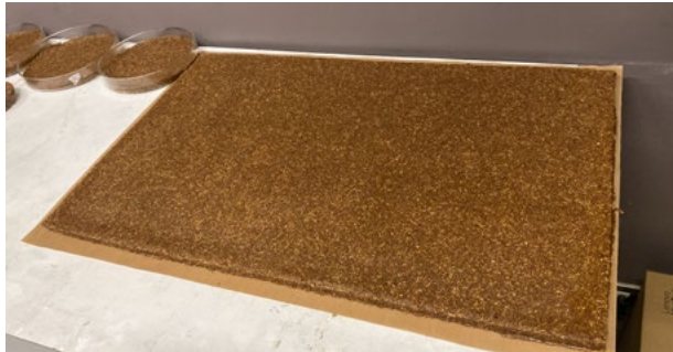
FIGURE 5. Composite panel made from a mixture of biopolymers and vegetable sawdust. The image shows the homogeneous integration of the components before molding and pressing.
