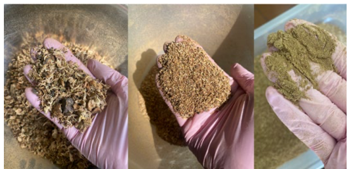
FIGURE 4. Grinding process. Uniform reduction of capsule particle size.
