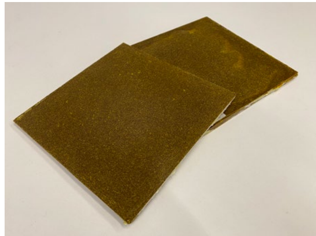
FIGURE 10. Final bio-agglomerated panel after thermal curing. Note the uniform surface, adequate compaction, and natural color of the material without chemical additives.
