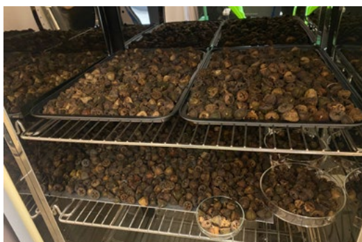
FIGURE 3. Drying process. Drying was conducted by evenly distributing the capsules in an oven to drive off internal moisture.
