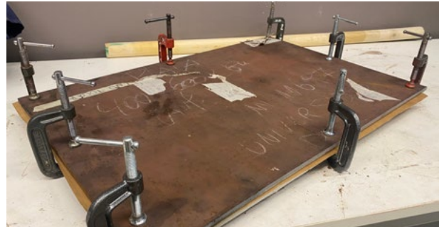
FIGURE 6. Experimental panels during the pressing process. The image shows the homogeneous compaction across the panel.
