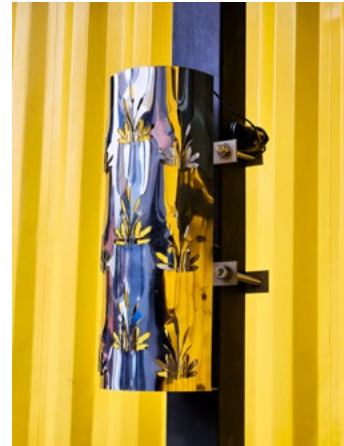
FIGURE 15. BIO-VASC. Acrylic and metal prototype measuring 50 x 18 x 18 cm. It contains a vertical aeration and lighting system. Source: photograph by Alexandra Huertas (December 7).
