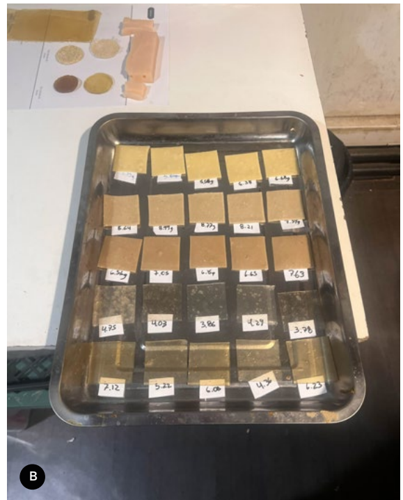
FIGURE 8A. Samples mixed for moisture content testing (own work), Figure 8B. Samples after moisture content measurement (own work).
