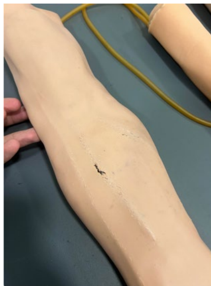
FIGURE 1. Breakage of the dermal layer due to accumulated punctures in phantoms used in practical exercises in nursing schools (own work).
